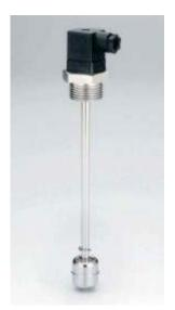
Top mount level switch with G1" (1"BSP) thread, enables this switch can be fitted to a tank through a G1" boss, without requiring access to the inside of the tank.
