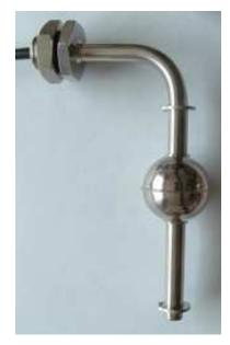
The SSV66-SM16 is a dual switch point side entry vertical float switch. This is mounted in a tank from the inside, so requires suitable access to the inside of the tank.
