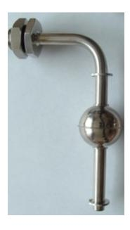
The SSV66-SPM12 is a dual switch point side entry vertical float switch. This is mounted in a tank from the inside, so requires suitable access to the inside of the tank.
