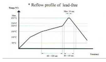
Recommendable reflow soldering condition as follows:
