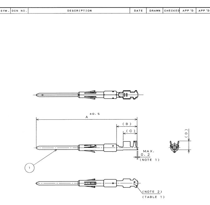
NOTE 1. NO PLATING ON THE SHEARED EDGES OF CONTACT.
