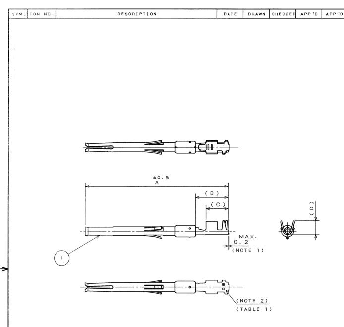
NOTE 1. NO PLATING ON THE SHEARED EDGES OF CONTACT.
