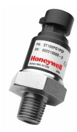
The Model ST pressure transducer combines Honeywell's proven silicon pressure sensing with the latest in ASIC technology in a rugged, industrial package. High value, coupled with outstanding performance, make this an ideal transducer for industrial control applications such as air compressors and pneumatic equipment. Temperature compensated, calibrated, and amplified, the ST has pressure ranges from 0 psi to 5.0 psi to 0 psi to 250 psi.
