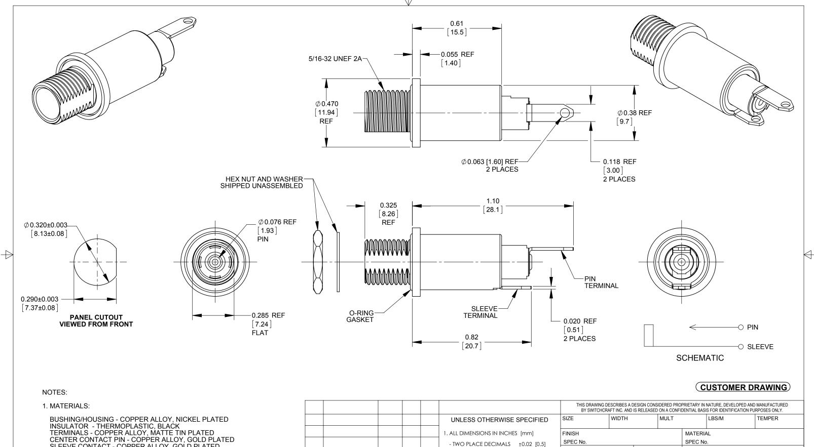
SLEEVE CONTACT - COPPER ALLOY, GOLD PLATED O-RINGS - THERMOPLASTIC RUBBER HEX NUT - COPPER ALLOY, NICKEL PLATED WASHER - STEEL, NICKEL PLATED
