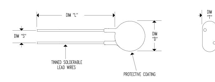
RESISTANCE @ +25°C = 16  $\Omega$  ± 20% MAXIMUM STEADY STATE CURRENT = 2 AMPS RESISTANCE @ Imax = 0.470  $\Omega$  NOMINAL
