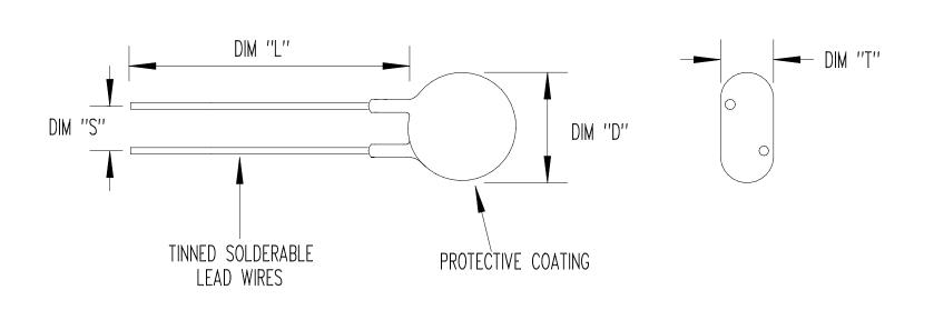
RESISTANCE @  $+25^{\circ}C = 20 \Omega \pm 20^{\circ}$
