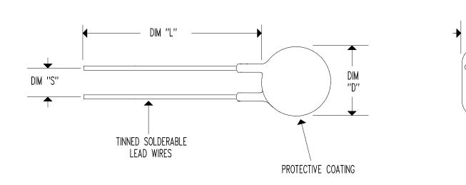
RESISTANCE @ +25 C = 25  $\Omega$   $\pm$  20% MAXIMUM STEADY STATE CURRENT = 2 AMPS RESISTANCE @ MAXIMUM CURRENT = 0.640  $\Omega$  NOMINAL
