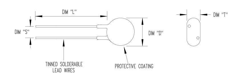
RESISTANCE @  $+25^{\circ}C = 2 \Omega \pm 20^{\circ}$
