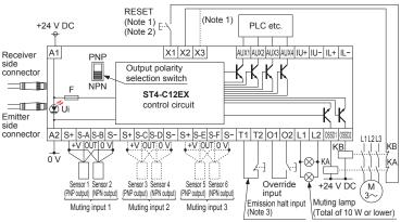
When using the normally open (NO) contact switch as a muting sensor, wire as shown in the figure below.
