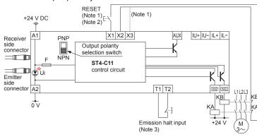
Notes: 1) The left diagram is when using manual reset. If automatic reset is used, disconnect the lead from X2 and connect it to X3. In this case, a reset (RESET) button is not needed.
