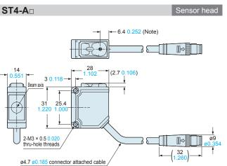
Note: It indicates the position of the emission amount adjuster on ST4-A□V.
