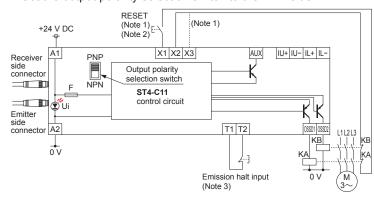
Notes: 1) The left diagram is when using manual reset. If automatic reset is used, disconnect the lead from X2 and connect it to X3. In this case, a reset (RESET) button is not needed.
