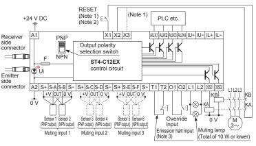
When using the normally open (NO) contact switch as a muting sensor, wire as shown in the figure below.
