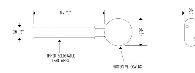
RESISTANCE @  $+25^{\circ}\text{C} = 5~\Omega~\pm~20\%$  MAXIMUM STEADY STATE CURRENT = 6 AMPS RESISTANCE @  $\text{Imax} = 0.135~\Omega~\text{NOMINAL}$
