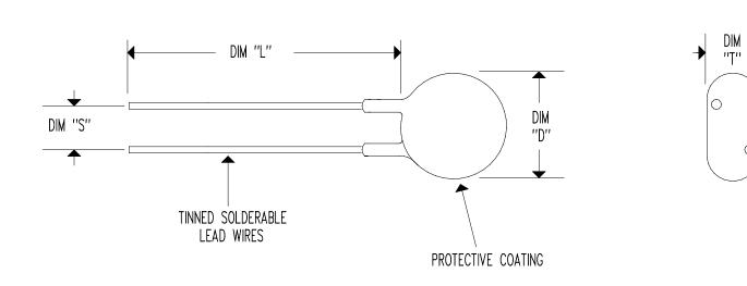
RESISTANCE @ +25'C = 5  $\Omega$  ± 20% MAXIMUM STEADY STATE CURRENT = 14 AMPS RESISTANCE @ MAXIMUM CURRENT = 0.060  $\Omega$  NOMINAL
