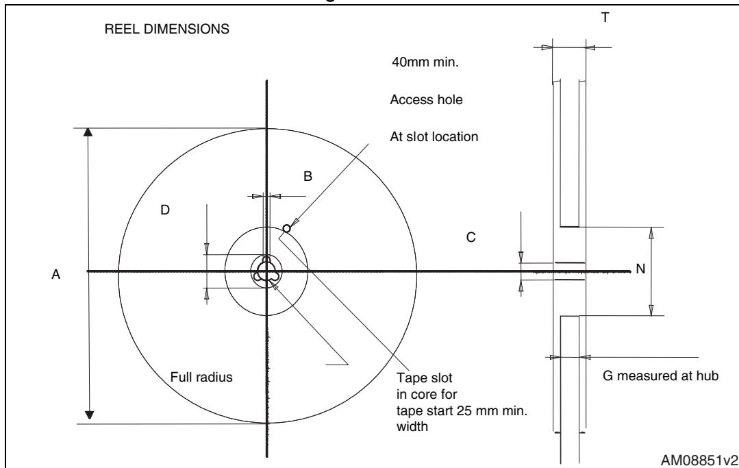
Table 12. D<sup>2</sup>PAK (TO-263) tape and reel mechanical data
