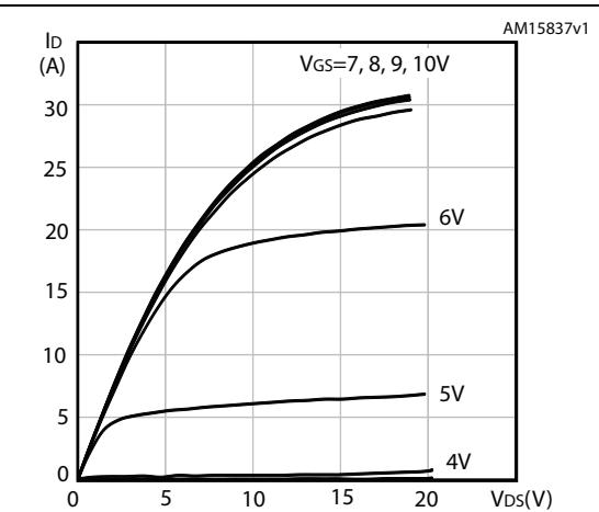
**Figure 6. Transfer characteristics**
