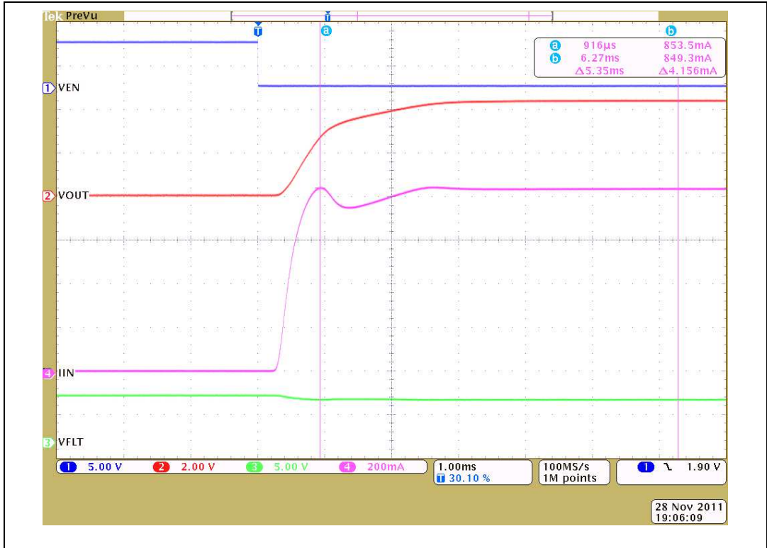
Figure 17. Soft-start performance for 100 \mu F capacitive load
