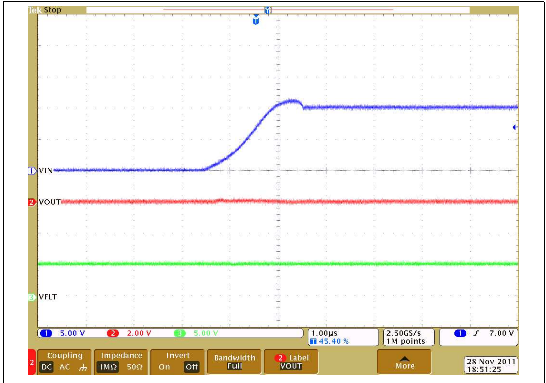
Figure 15. Startup to overvoltage (detail)
