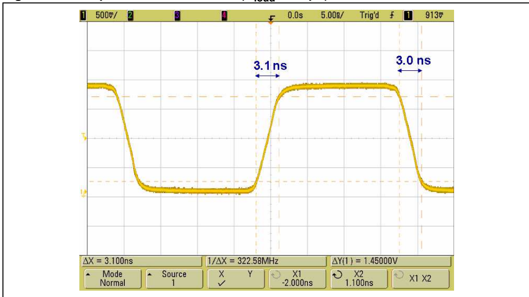
Figure 20. Output clock rise/fall time ( C_{load} = 40\text{ pF} )
