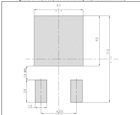
Figure 20: DPAK (TO-252) recommended footprint (dimensions are in mm)
