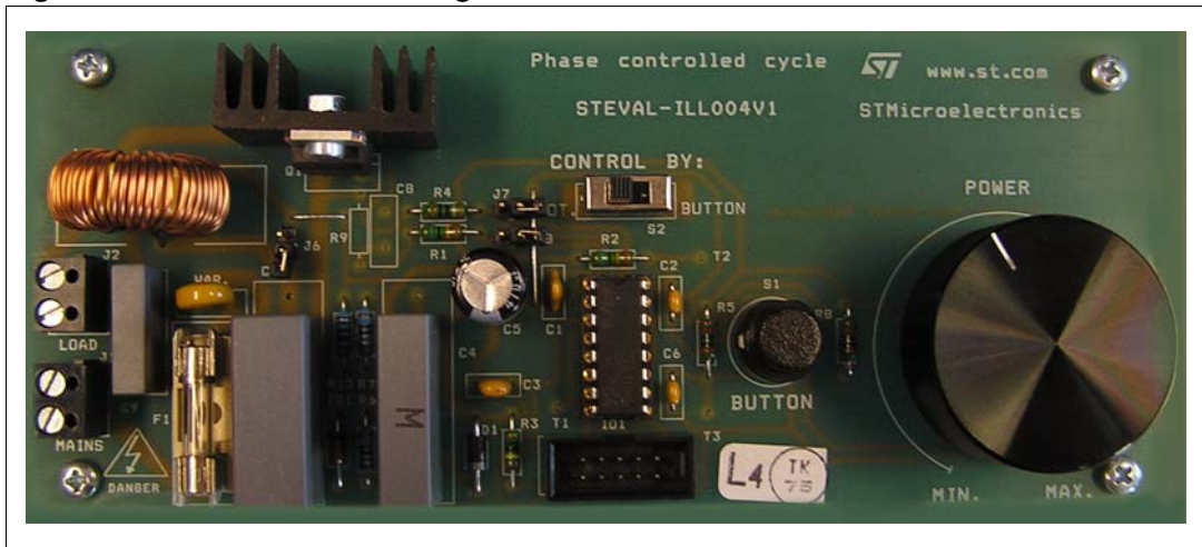
Figure 10. STEVAL-ILL004V1 light dimmer evaluation board
