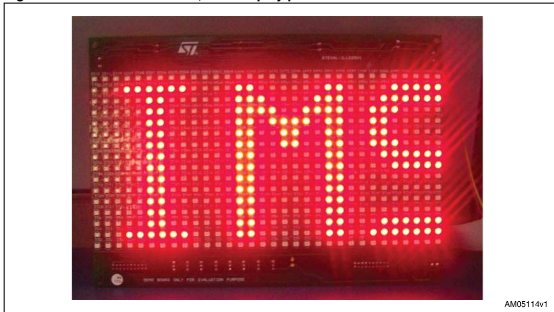
Figure 1. STEVAL-ILL025V1, LED display panel
