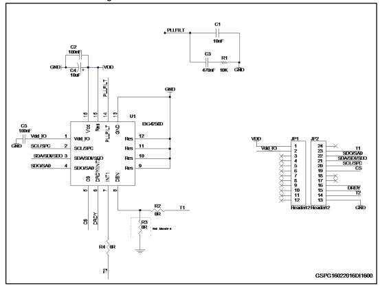
Figure 1: STEVAL-MKI169V1 schematic circuit
