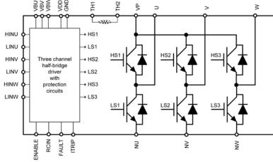
Figure 1. Functional Diagram
