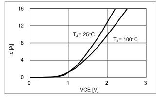
Figure 4. V<sub>CE</sub> versus ID for different temperatures  $(V_{DD} = 15 V)$
