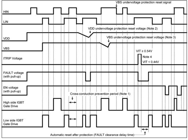
Figure12. Input/Output Timing Chart
