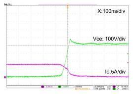
Figure 11. Turn-off waveform Tj = 100°C, V<sub>CC</sub> = 400 V
