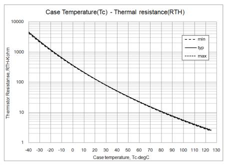
Figure13. Thermistor Resistance versus Case Temperature
