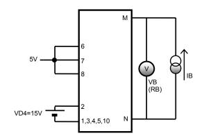
Figure 20. Test circuit for RB
