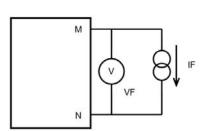
Figure 19. Test circuit for VF
