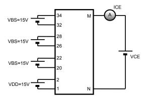
Figure 17. Test Circuit for ICE
