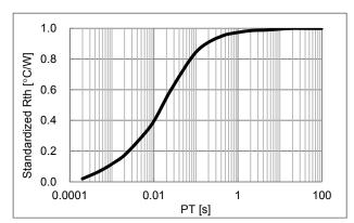
Figure 8. Thermal impedance plot (IGBT)
