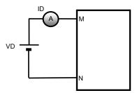
Figure 21. Test circuit for ID
