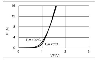
Figure 5. V<sub>F</sub> versus ID for different temperatures
