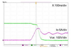
Figure 10. Turn-on waveform Tj = 100°C, V<sub>CC</sub> = 400 V
