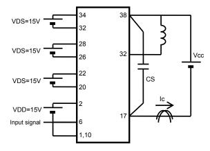
Figure 22. Switching time test circuit
