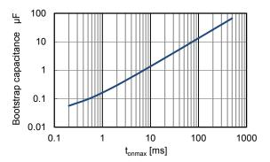
Figure 15. Bootstrap capacitance versus tonmax
