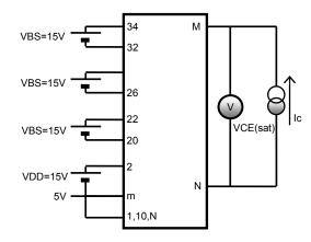
Figure 18. Test circuit for VCE(sat)
