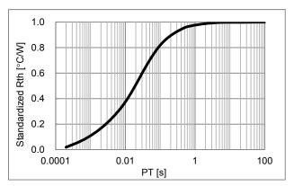
Figure 9. Thermal impedance plot (FRD)
