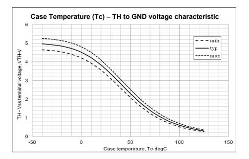
Figure 14. Thermistor Voltage versus Case Temperature Conditions : RTH = 39 k $\Omega$ , pull-up voltage 5.0 V (see Figure 2)
