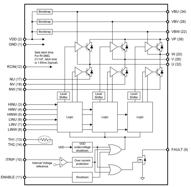
Figure 3. Simplified Block Diagram
