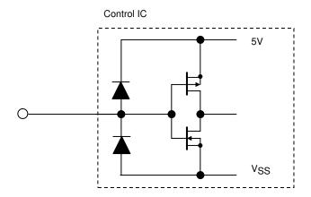
All input pins of this driver support schmitt input. Typ specifications at Tc = 25°C are given below. Hysteresis voltage is 0.6V (VIHa-VILa).
