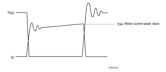
Figure 2 Output Current, I<sub>D</sub>, and Voltage, V<sub>DS</sub>, Waveforms 2 of the STK672-5\*\* Series when Driving a 2-Phase Stepping Motor with Constant Current Chopping
