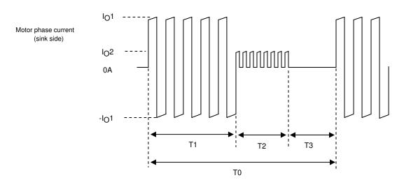
Figure 1 Motor Current Timing
