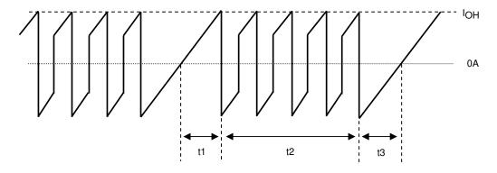
Motor COM Current Waveform Model
