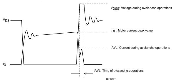
Figure 1 Output Current, ID, and Voltage, VDS, Waveforms 1 of the STK672-5\*\* Series when Driving a 2-Phase Stepping Motor with Constant Current Chopping
