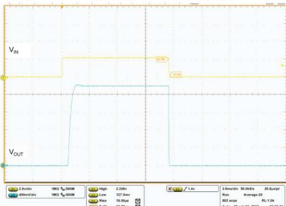
**Figure 33: Startup transient**
