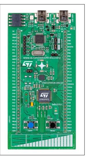
Based on the STM32F072RBT6, it includes an ST-LINK/V2 embedded debug tool interface, an ST MEMS gyroscope, LEDs, push-buttons, Linear touch sensor, touchkeys, RF EEPROM connector and a USB mini-B connector.
