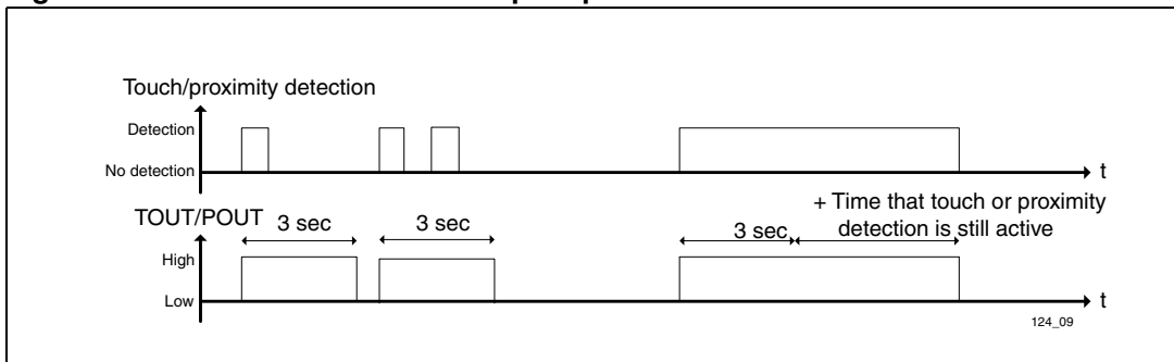
Figure 14. 3-second latch mode output operation
