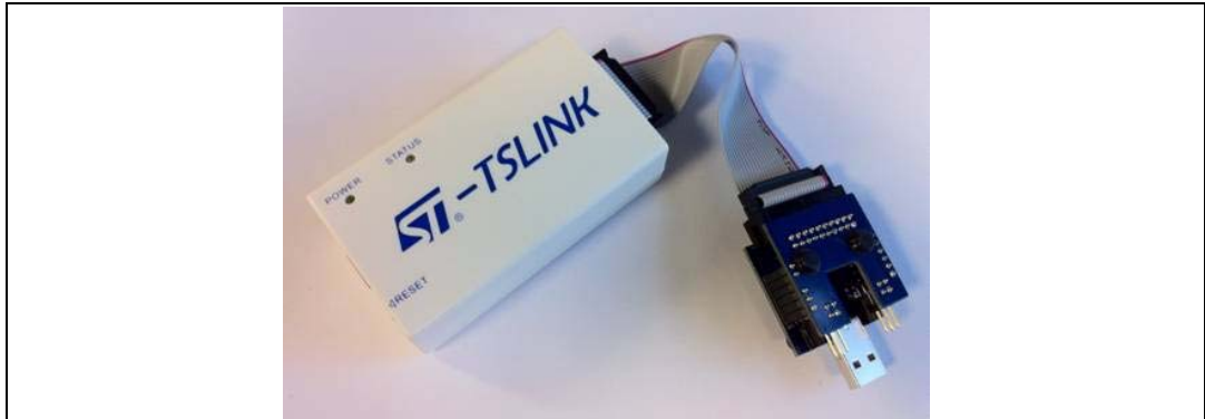
Figure 11. MB973/MB972 board assembly connected to ST-TSLINK dongle
