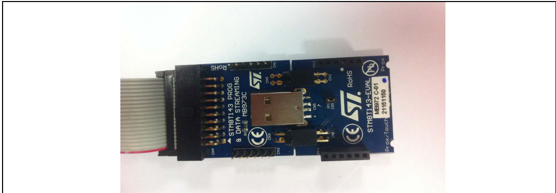
Figure 14. Connectors MB972 CN1-CN2 connected to connectors MB973 CN3-CN5
