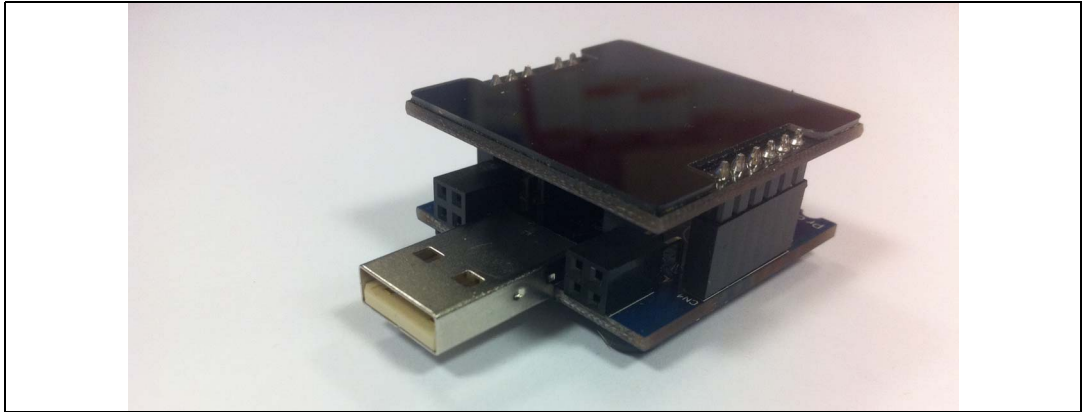
Figure 2. MB976 electrode board connected to MB972 controller board
