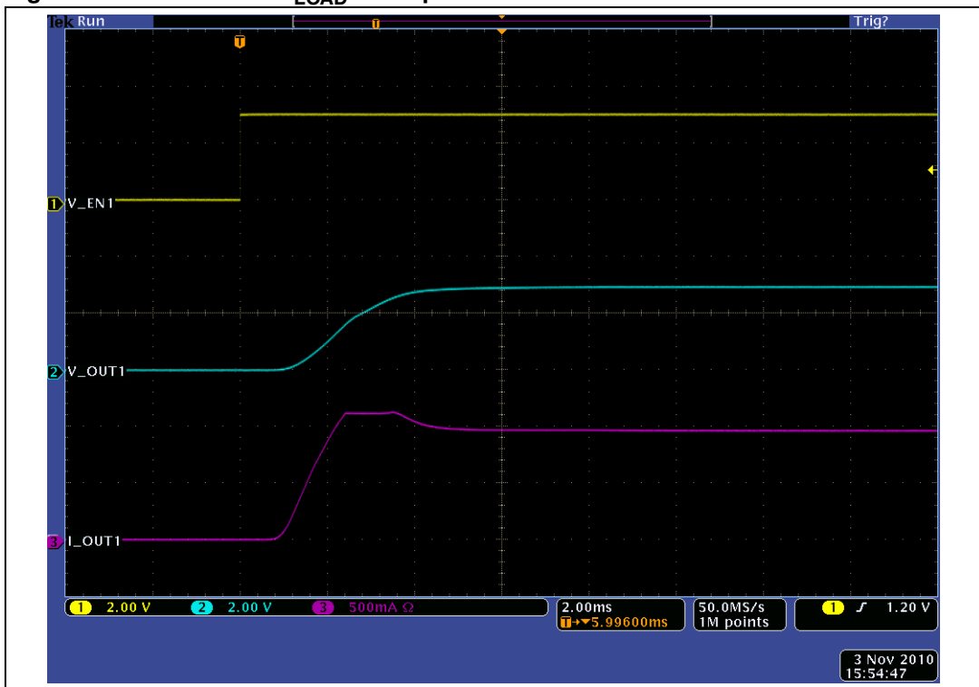
Figure 25. Turn-on for C_{LOAD} = 470 \mu F
