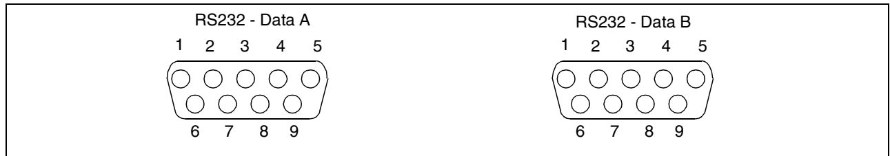
Figure 9: RS232 transmit and receive connectors: CN7, CN8
