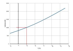
**Remark:** Values of electric resistance correspond almost exactly to KTY83. Above140°C the sensor may loose its linearity.
