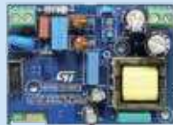
STEVAL-ILL082V1/ STEVAL-ILL083V1 Smart home lighting based on HVLED815PF and SPSGRF (STEVAL-ILL082V1) and SPBTLE-RF (STEVAL-ILL083V1)
