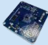
STEVAL-ISB036V1 Wireless charger receiver based on STWLC03
