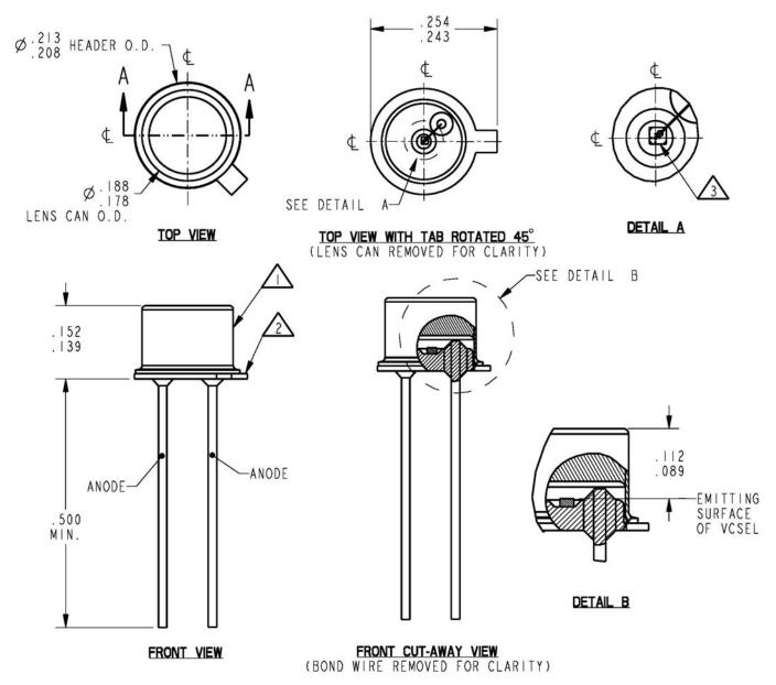
MOUNTING DIMENSIONS (for reference only): All dimensions are in inches. [mm]
