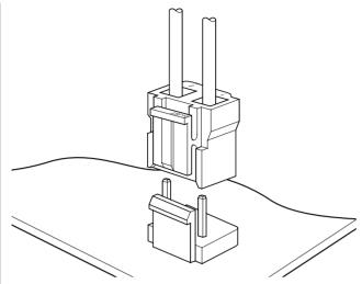
This 7.92mm pitch large current carrying capacity connector is used with primary power supply circuits and various other circuits requiring large currents. It features an anti-misinsertion construction and a reliable locking mechanism to ensure maximum safety.
