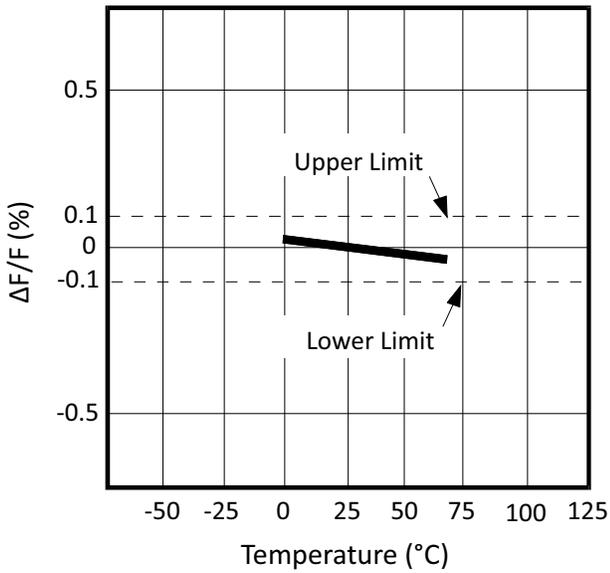
Figure 5: %  $\Delta$  Freq. vs. Temperature (SWR200M)
