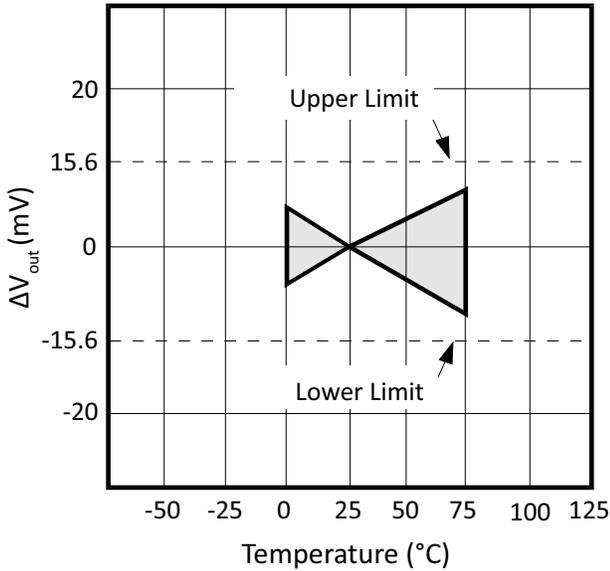
Figure 3:  $V_{OUT}$  vs. Temperature (SWR200M)
