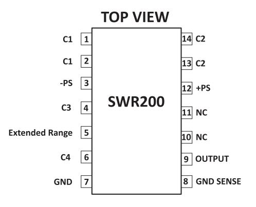
Figure 13: Pin Configuration
