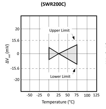
Figure 2: V<sub>OUT</sub> vs. Temperature
