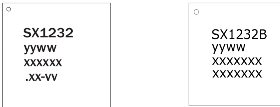
Figure 3. Marking Diagram SX1232 & SX1232B
