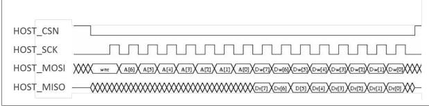
Figure 3: SPI Timing Diagram (Single Access)
