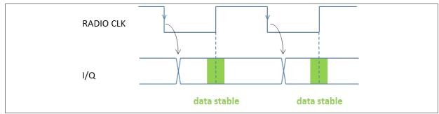
Figure 5: I/Q on Clock Falling Edge
