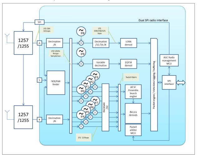
Figure 12: Dual Band Operation
