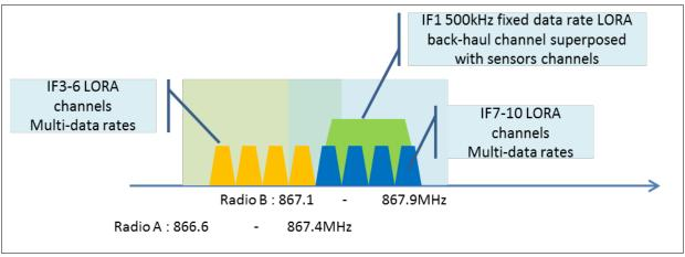
Figure 10 Radio Spectrum
