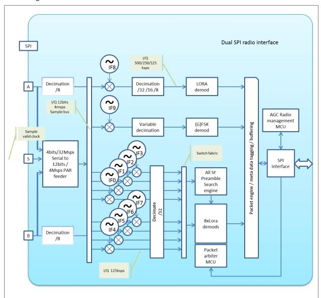
Figure 6: SX1301 Digital Baseband Chip Block Diagram
