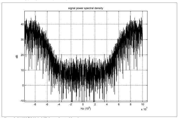
Figure 8: SX1255/57 Digital I/Q Power Spectral Density
