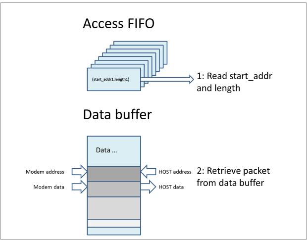
Figure 7: Access FIFO and Data Buffer
