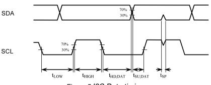
Figure 5 I2C Data timing
