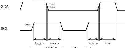
Figure 4 I2C Start and Stop timing
