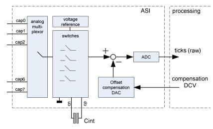
Figure 17 Analog Sensor Interface
