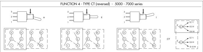
Single pole switches in a double pole case Double pole switches in a four pole case
