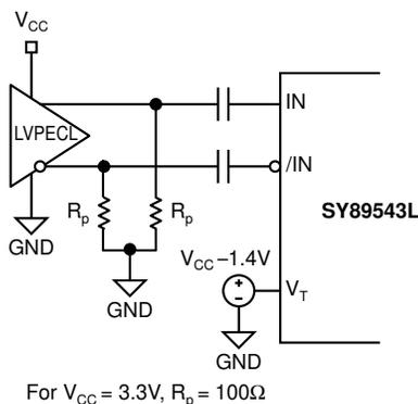
For  $V_{CC} = 3.3V$ ,  $R_p = 100\Omega$
