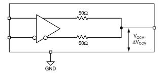
Figure 5b. LVDS Common Mode Measurement
