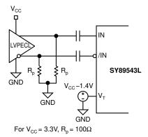
Figure 4d. LVPECL Interface (AC-Coupled)
