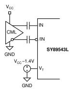
Figure 4b. CML Interface (AC-Coupled)
