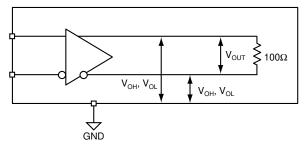
Figure 5a. LVDS Differential Measurement
