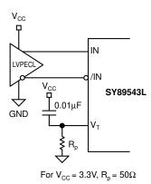
Figure 4c. LVPECL Interface (DC-Coupled)
