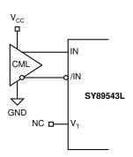
Figure 4a. CML Interface (DC-Coupled)
