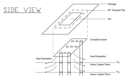
PCB Thermal Consideration for 32-Pin MLF® Package (Always solder, or equivalent, the exposed pad to the PCB)
