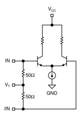
Figure 3. Simplified Differential Input Stage
