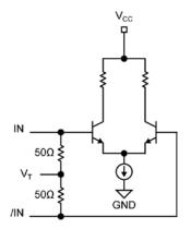
Figure 3a. Simplified Differential Input Stage
