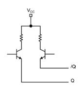
Figure 3b. Simplified LVPECL Output Stage
