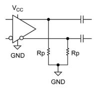
Note: For +2.5V systems:  $Rb = 50\Omega$ For 3.3V systems  $Rb = 100\Omega$ The output pair requires a DC-current path to GND.
