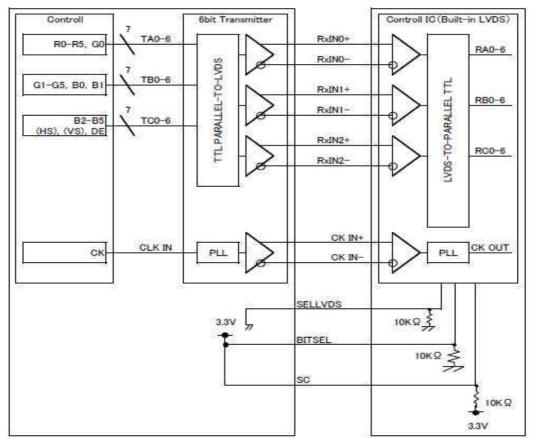
$\mbox{\ensuremath{\mbox{\$}}}\mbox{SELLVDS}$  signal line has 10 k  $\Omega$  -pulldown resister.
