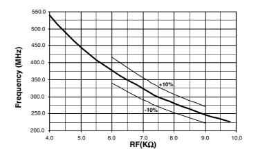
**Figure 9-2.** Oscillator Swing versus Resistor RS (RF =  $7.5 \text{ k}\Omega$ )
