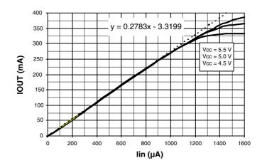
**Figure 9-5.** Voltage Compliance R (IOUT to VCC) =  $5.9\Omega$
