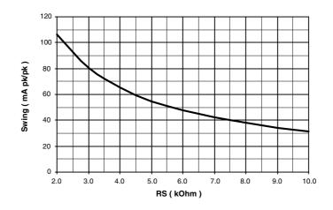
Figure 9-3. Oscillator Frequency Dependency of Swing
