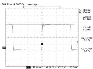
Figure 9-6. Step Response, Read Channel: 50 mA, Channel 2: 50 mApp
