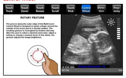
The MTCW touchpad has a unique indented outer ring. Sliding one finger inside this circular indentation can be recognized as a unique gesture. This
