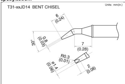
NOTE:  $xx:00 = 480^{\circ}C (895^{\circ}F) | 01 = 450^{\circ}C (840^{\circ}F) | xx:02 = 400^{\circ}C (750^{\circ}F) | xx:03 = 350^{\circ}C (660^{\circ}F)$
