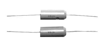
The Type TAC molded solid tantalum capacitor is great for putting a lot of capacitance in a small space in a high temperature application. The TAC is constructed in a shock and vibration resistant, flame retardant, rugged, precision molded case that is tapered on one end for polarity identification and available on tape and reel.
