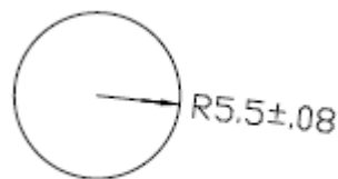
Recommended panel hole cutout (mm)
